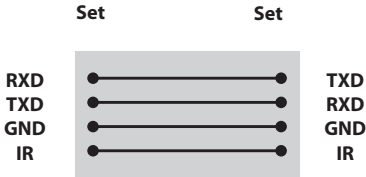
4-Wire Configurations (Standard RS-232C cable)
